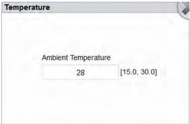
You can view the current ambient temperature of the analyzer. If the results of the temperature testing exceed the normal range, they will be highlighted by the red background.
