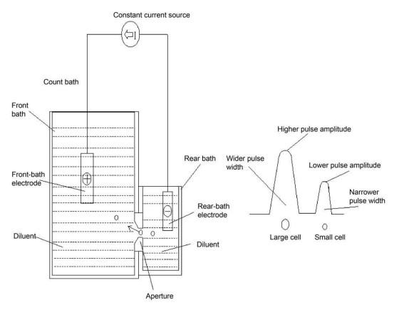
Figure 4-3 Electrical Impedance method
