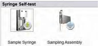
3. Double click the part that needs to be tested, e.g. **Sample Syringe**, and wait for the self-inspection results.
