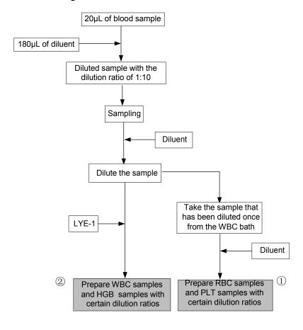
Figure 4-2 Dilution Procedures in Predilute Mode
