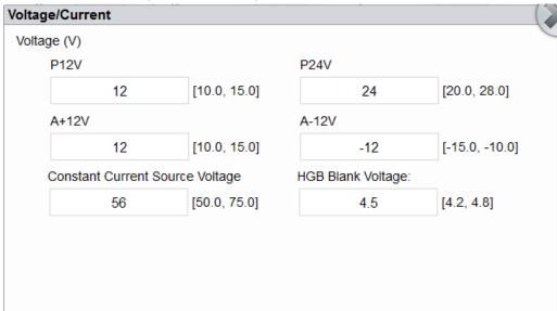
You can view the voltage and current information of the analyzer. The voltage or current value that exceeds the normal range will be displayed in a red background.
