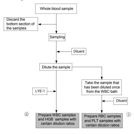
Figure 4-1 Dilution Procedures in Whole-Blood Mode
